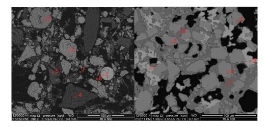
Figure 6 Mineralogical analysis data of raw and reduced BREX sample with Alcotac®CB6. Left - raw BREX (1-iron, 2-magnetite, 3-calcium ferrite,  $4-SiO_2$ , 5-CaO, 6-tridymite, 7-carbon); on the right - reduced briquette at a temperature of 1100 °C (1,2 - iron, 3,5 - Hematite, 4 - magnetite, 6,7 – olivine)
