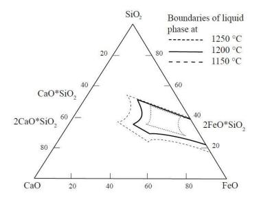
Figure 8 Phase diagram of CaO- FeO- SiO<sub>2</sub>
