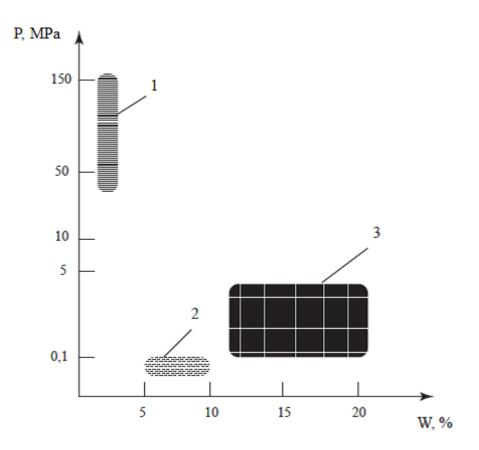
Figure 1 Comparison of technologies of briquetting according to the parameters of briquetting (applied pressure P and moisture content of the charge W). 1 - roller pressing, 2 - vibropressing, 3 – stiff vacuum extrusion
