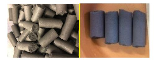
Figure 11 Green (left) and fired Magnetite BREX
