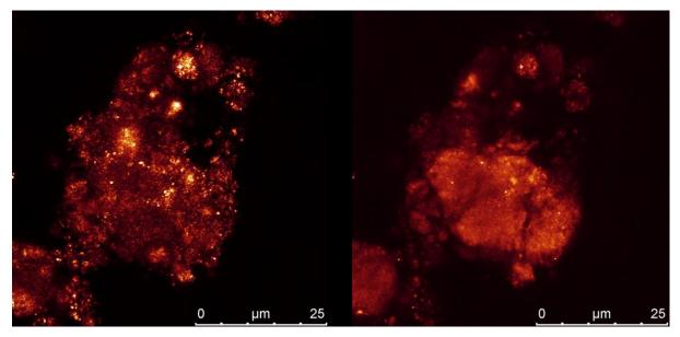
Figure 3. Confocal Laser Scanning Microscopy (CLSM) images of bentonite suspension with Alcotac® CS polymer binder added. Left: reflected light. Right: emitted fluorescence.
