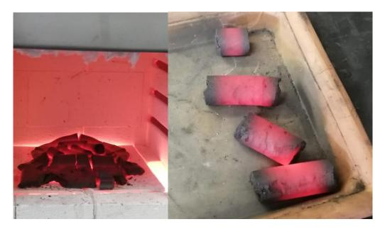
Figure 12 Appearance of the BREX during thermal stability testing (left) and after extraction from the furnace
