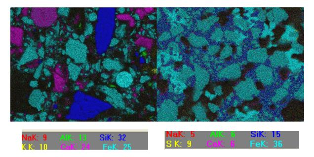
Figure 7 Raw (left) and reduced samples. Image combined in the characteristic radiation of the elements
