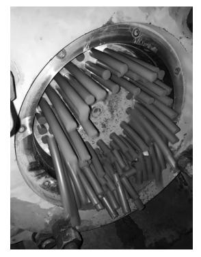
Fig. 8.25 Industrial production of chromium-based brex at Aktobe Ferroalloy Plant Aktobe Ferro Alloys Plant Report on BREX Smelting
